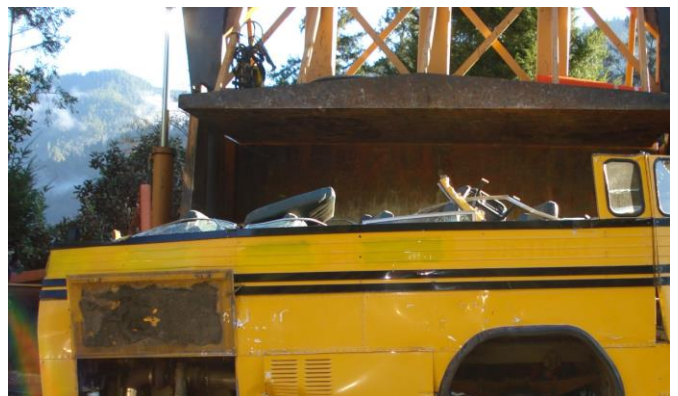
Example of acceptable destruction of vehicle chassis
