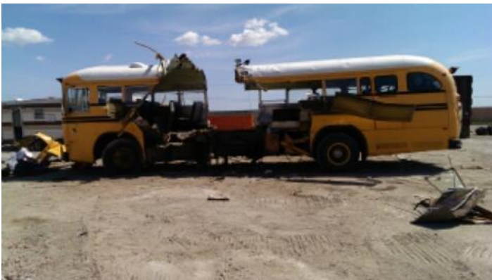
Example of acceptable destruction of vehicle chassis
